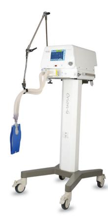
A ventilator is a life-saving equipment. This means that ICU staffs need real-time information in order to make the right decision. The Orion-G comes with a 7" TFT colour touch-screen that can display up to 4 curves, along with a host of monitored parameters. Also its highly responsive touch-screen and its encoder knob helps you choose and set your parameters in a safe, quick and easy way.
